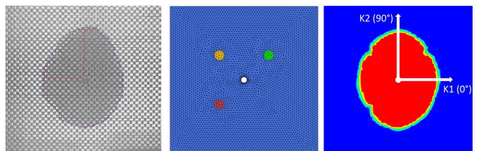
Figure 3: Test view (left), fabric layer with resistive welding zones (green, yellow, red) (middle), numerical flow front (right)
